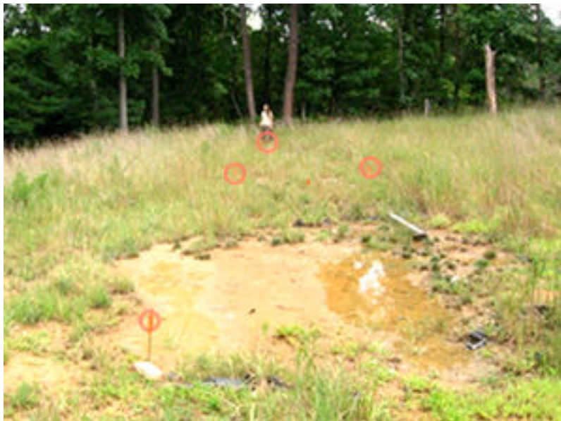
Photograph 1. View of the pit area showing perimeter of exposed black plastic (indicated by red circles). Molly is standing at easternmost edge of perimeter about 100 feet away. Sparsely vegetated area with highest chloride tests is in foreground. Photograph was taken looking east.
